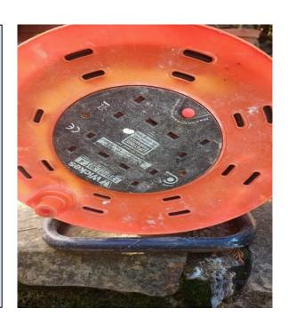
In the event of overload, it would be hoped that the fuse will blow and power will be lost to the affected circuit, but this does not always occur with slight overload. Fuses are designed to operate (fail or blow) quickly with a significant overload, sometimes called a short-circuit, and also to continue to operate over a period of time with a small overload to the circuit.
